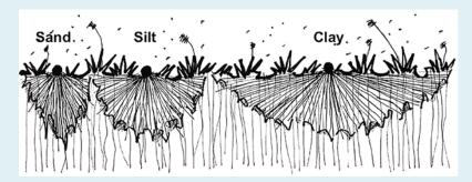
Type of soil greatly impacts the amount of water needed and its horizontal spread. Irrigating 1 square foot to 4" deep requires 0.205 gallons of water in sandy soils, 0.300 in silty soils, and 0.415 in clay soils.
