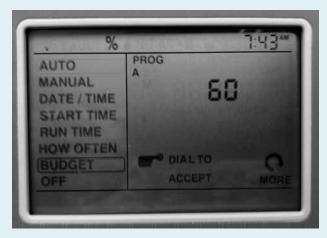
The budget adjustment feature on your automatic irrigation controller is a quick way to respond to changing conditions. Mid-summer monsoon? Reduce all irrigation by 60%. June gloom in July? Reduce all irrigation by 40%. Budget adjustment allows for quick control of all irrigation valves.
