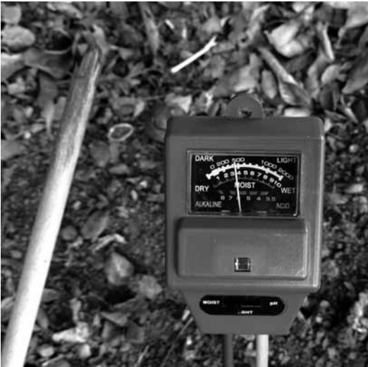
Despite the soil looking dry both the moisture meter and wooden dowel indicate that there is plenty of moisture 4" down.
