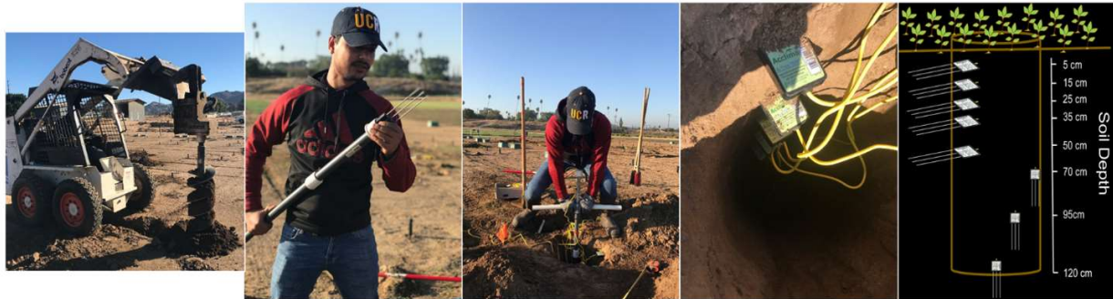
Figure 2. TDR sensors installation steps at different depths.
