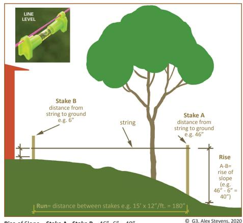
**Rise** of Slope = **Stake A** - **Stake B** = 46"- 6" = 40" **Run** of Slope = 180"
