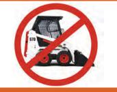
The bigger the equipment for removing the turf, the more the soil beneath is compacted. Try to only use hand powered or walk-behind equipment rather than a bobcat or other scraper.
