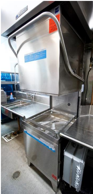
Figure 15: Meiko DV80.2 WAHRS as installed at The Counter
