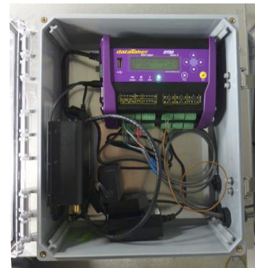
Figure 6: Enclosure with data logger and cell modem
