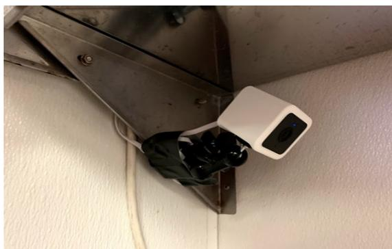
**Figure 2:** Camera mounted onto the corner strut.
