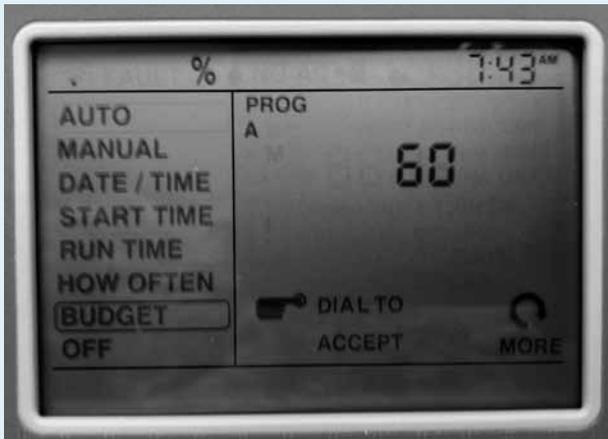
The budget adjustment feature on your automatic irrigation controller is a quick way to respond to changing conditions. Mid-summer monsoon? Reduce all irrigation by 60%. June gloom in July? Reduce all irrigation by 40%. Budget adjustment allows for quick control of all irrigation valves.
