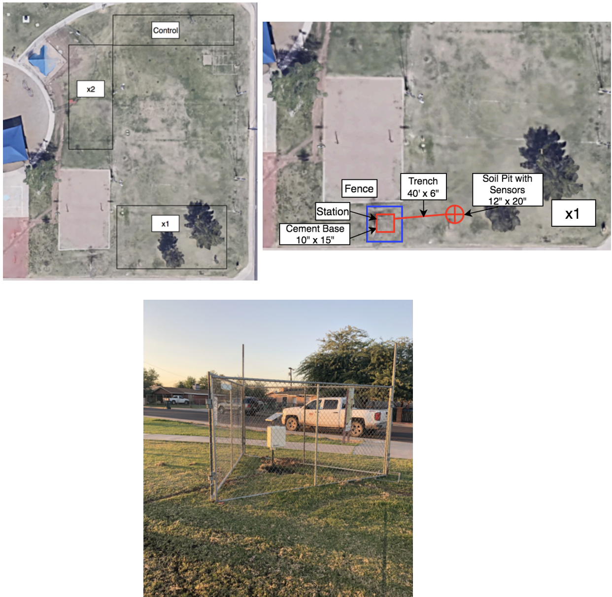
Figure 5. Study site location at Smith Park (top) with control and treatment plots. Photograph of fenced soil moisture station (bottom), which includes a solar panel, datalogger, rain gauge, and soil moisture sensors at multiple depths.
