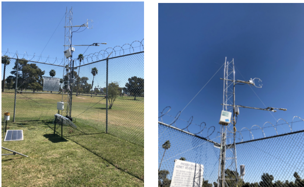
Figure 15. Photograph of complete eddy covariance system (left) that includes sonic anemometer, infrared gas analyzer, net radiometer, rain gauge, datalogger, soil moisture sensors, thermocouple sensors and solar panels. Primary instruments for eddy covariance system (right).
