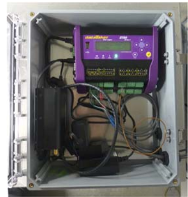
Figure 2. Enclosure with data logger and cell modem
