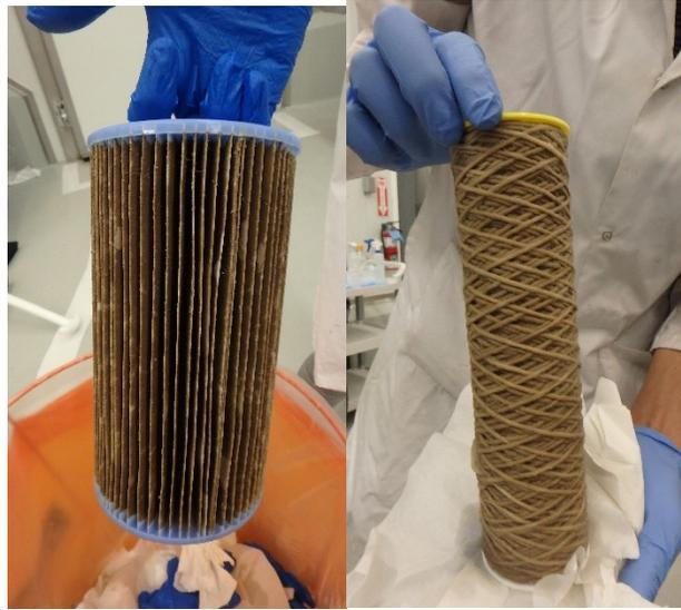
*Figure 14: 50-micron filter post treatment (left) and 5-micron filter post treatment (right)*
