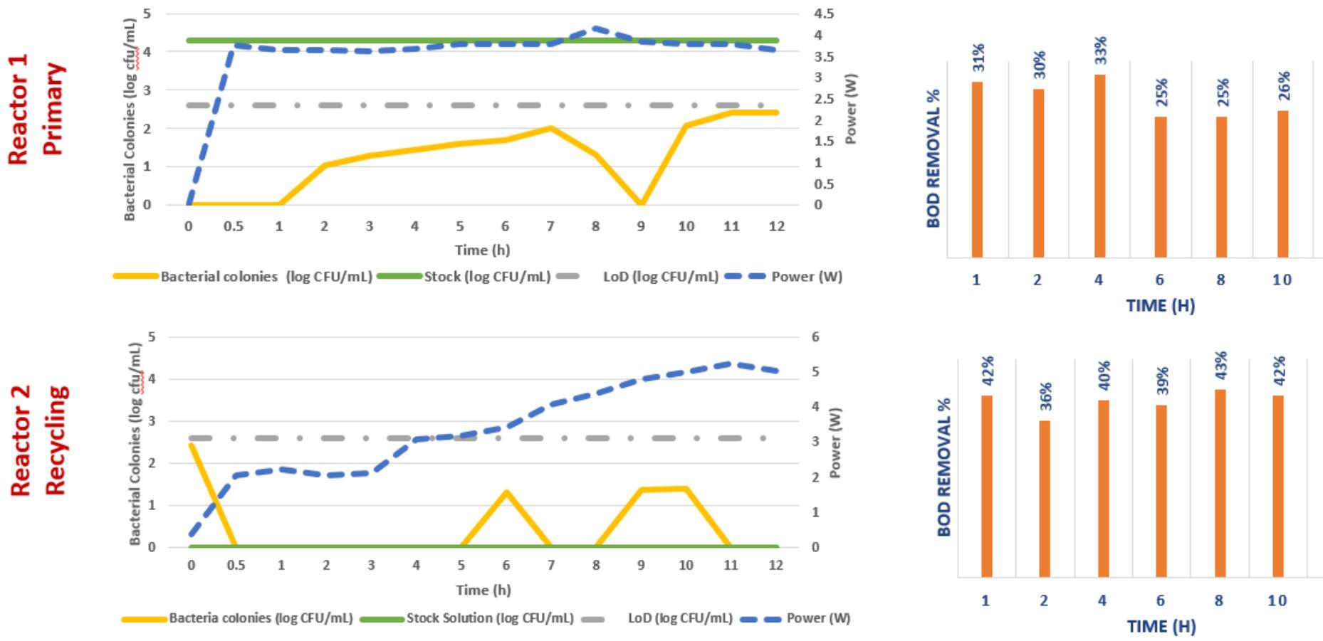
Figure 9: Bacterial inactivation and BOD removal in chill tank water using two 2" reactors in series at 80 mL/min, 8V and 20 ppm KI.
