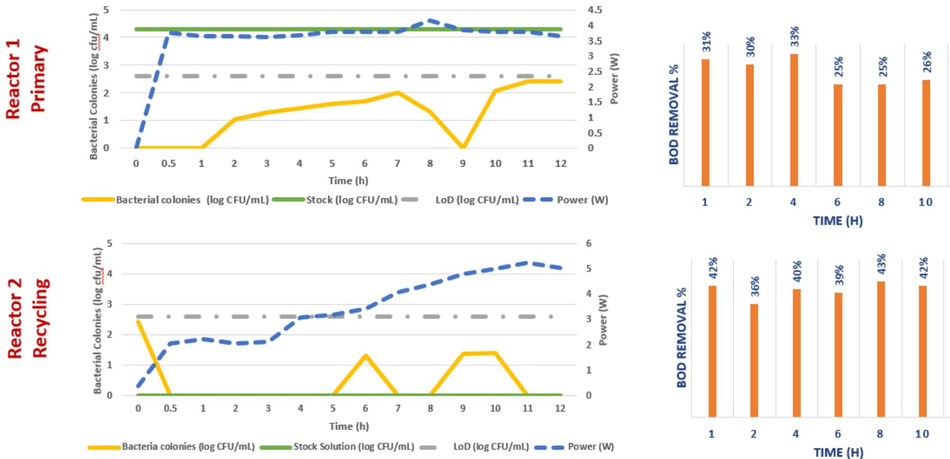
Figure 9: Bacterial inactivation and BOD removal in chill tank water using two 2" reactors in series at 80 mL/min, 8V and 20 ppm KI.
