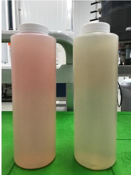
*Figure 10: Chill tank stock (left) and post AOS treatment (right).*
