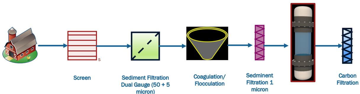
Figure 11: Proposed Treatment Train for Poultry Waste Water.
