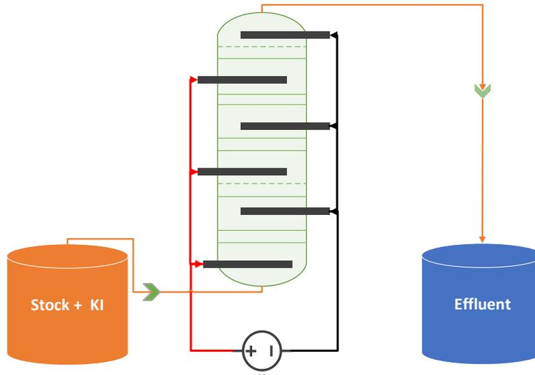
Figure 5: 2"- 6 chamber reactor experimental setup.
