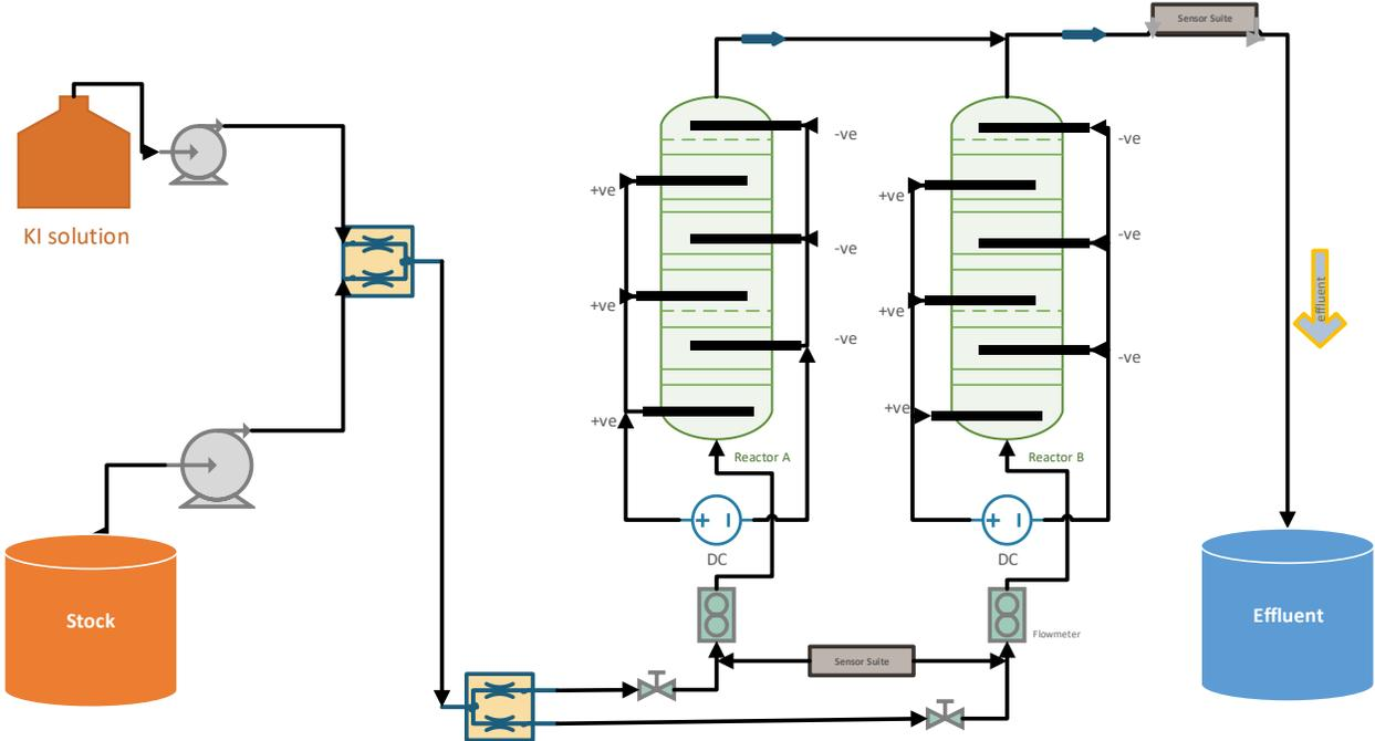
Figure 6: 2"- 6 chamber reactor experimental setup.
