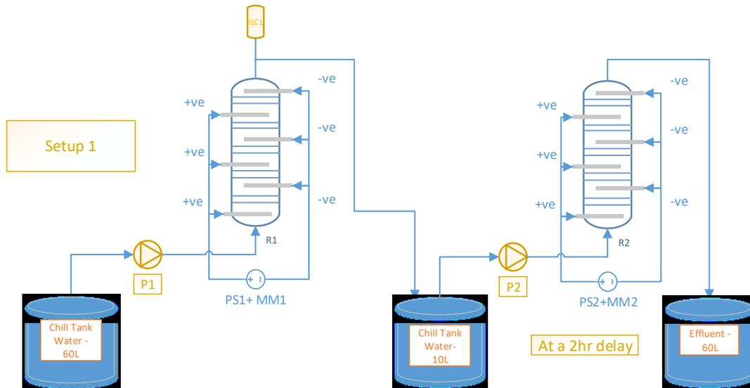
Figure 7: 2"- 6 chamber reactor in series experimental setup.
