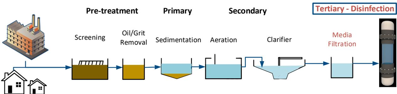
Figure 15: Generic municipal wastewater treatment plant with the AOS as the tertiary treatment step.
