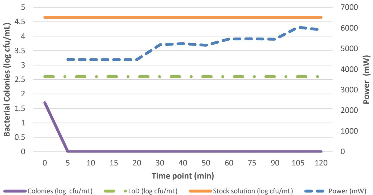
Figure 8: Bacterial inactivation in chill tank water using the AOS 2" reactor at 80 mL/min, 8V and 20 ppm KI.
