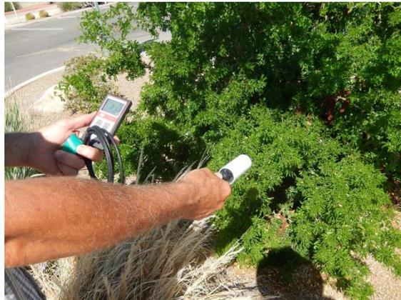
Fig. 3. Collecting data to develop new schedule before the test was started (left) and collecting infrared temperatures of a tree canopy (right).
