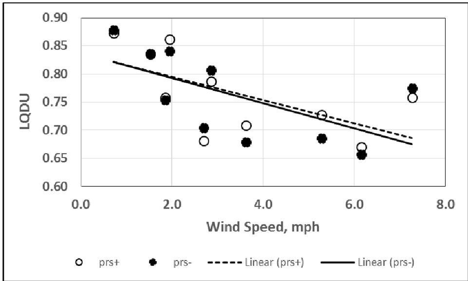
Figure 16. Low quarter mean distribution uniformity (LQDU) plotted as a function of wind speed for plots irrigated with prs- and prs+ rotors at system operating pressure of 60 psi. Regression lines relating LQDU to wind speed are plotted if the line slopes are significantly different from zero.
