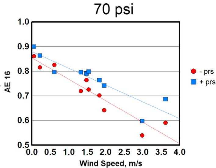
Figure 8. Application efficiency computed using the 16 interior catch cans (AE16) plotted as a function of wind speed during system operation for plots irrigated with (+prs) and without (-prs) pressure regulation when line pressure was set at 70 psi.
