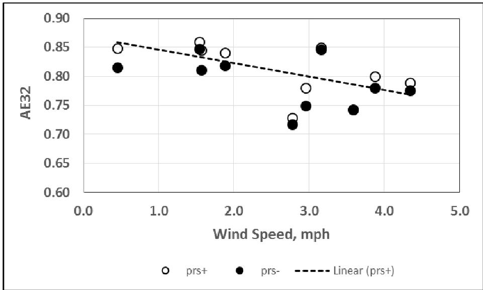
Figure 12. Application efficiency as determined from all 32 catch cans (AE32) plotted as a function of wind speed for plots irrigated with prs- and prs+ rotors at system operating pressure of 45 psi. Regression lines relating AE32 to wind speed are plotted if the line slopes are significantly different from zero.
