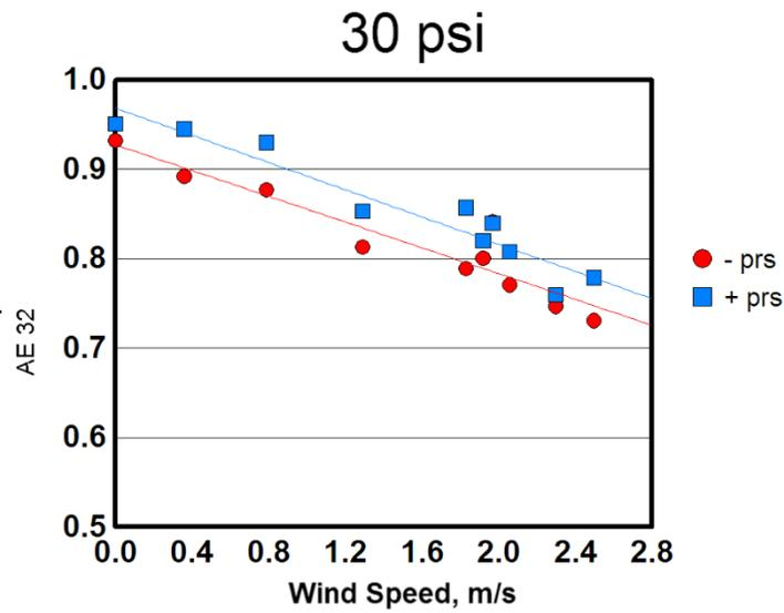
Figure 3. Application efficiency computed using all 32 catch cans (AE32) plotted as a function of wind speed during system operation for plots irrigated with (+prs) and without (-prs) pressure regulation when line pressure was set at 30 psi.
