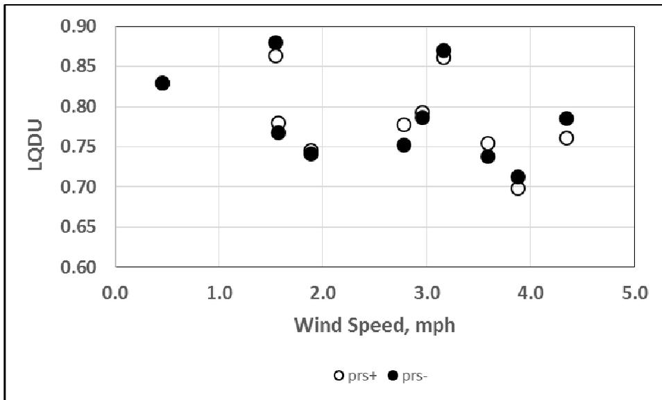
Figure 15. Low quarter mean distribution uniformity (LQDU) plotted as a function of wind speed for plots irrigated with prs- and prs+ rotors at system operating pressure of 45 psi. Regression lines relating LQDU to wind speed are plotted if the line slopes are significantly different from zero.
