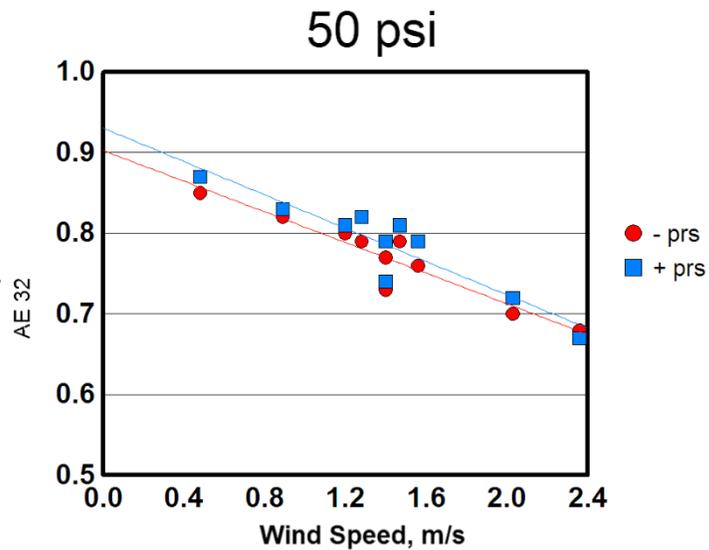
Figure 6. Application efficiency computed using all 32 catch cans (AE32) plotted as a function of wind speed during system operation for plots irrigated with (+prs) and without (-prs) pressure regulation when line pressure was set at 50 psi.
