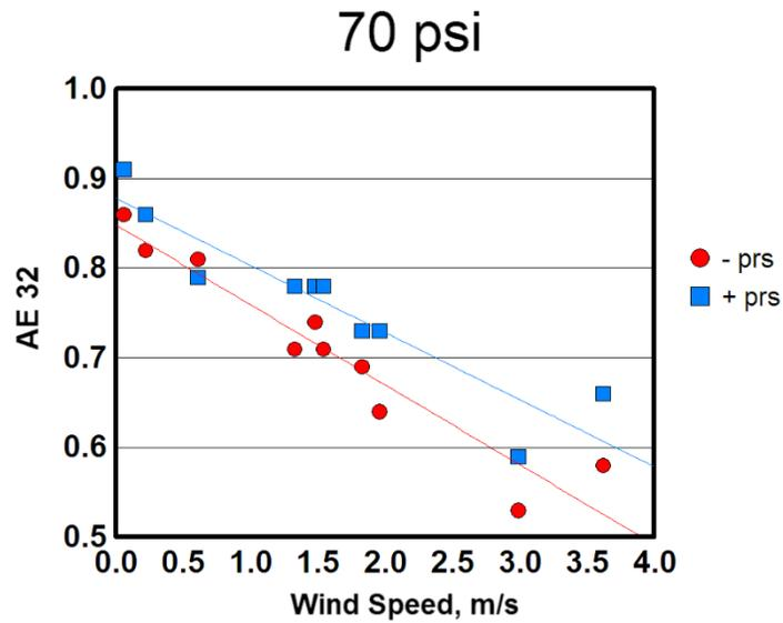
Figure 9. Application efficiency computed using all 32 catch cans (AE 32) plotted as a function of wind speed during system operation for plots irrigated with (+prs) and without (-prs) pressure regulation when line pressure was set at 70 psi.
