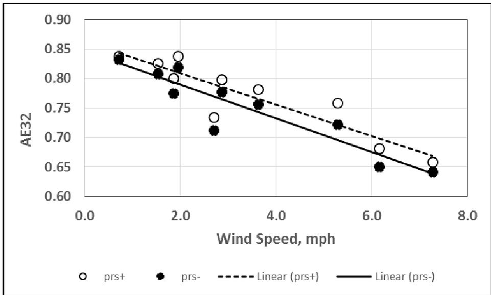
Figure 13. Application efficiency as determined from all 32 catch cans (AE32) plotted as a function of wind speed for plots irrigated with prs- and prs+ rotors at system operating pressure of 60 psi. Regression lines relating AE32 to wind speed are plotted if the line slopes are significantly different from zero.
