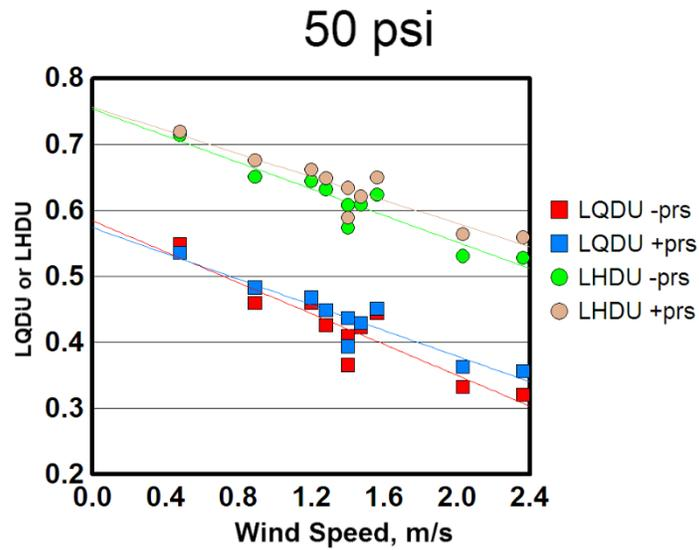
Figure 7. Low quarter distribution uniformity (LQDU) and low half distribution uniformity (LHDU) plotted as a function of wind speed during system operation for plots irrigated with (+prs) and without (-prs) pressure regulation when line pressure was set at 50 psi.
