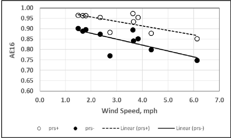
Figure 11. Application efficiency as determined from the 16 internal catch cans (AE16) plotted as a function of wind speed for plots irrigated with prs- and prs+ rotors at system operating pressure of 75 psi. Regression lines relating AE16 to wind speed are plotted if the line slopes are significantly different from zero.
