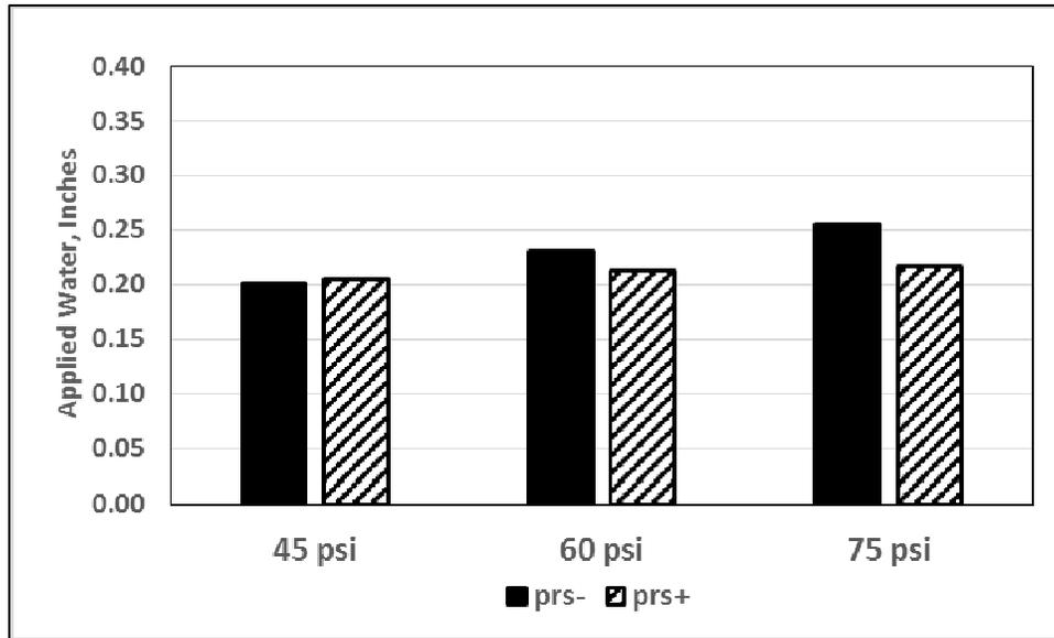
Figure 4. Depth of water applied to plots irrigated with prs- and prs+ rotors at system operating pressures of 45, 60 and 75 psi. Depth measured using the both interior and perimeter catch cans.
