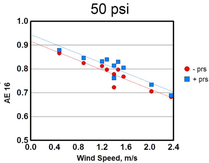
Figure 5. Application efficiency computed using the 16 interior catch cans (AE16) plotted as a function of wind speed during system operation for plots irrigated with (+prs) and without (-prs) pressure regulation when line pressure was set at 50 psi.
