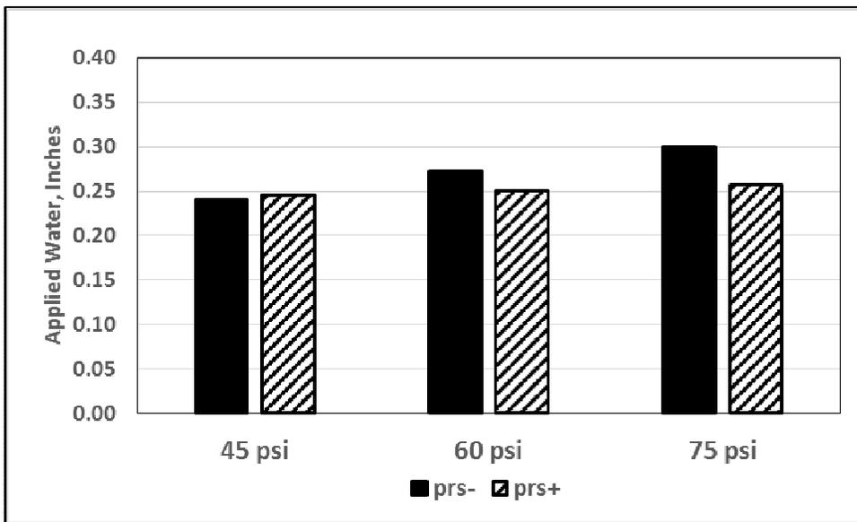
Figure 3. Depth of water applied to plots irrigated with prs- and prs+ rotors at system operating pressures of 45, 60 and 75 psi. Depth measured using the 16 interior catch cans.
