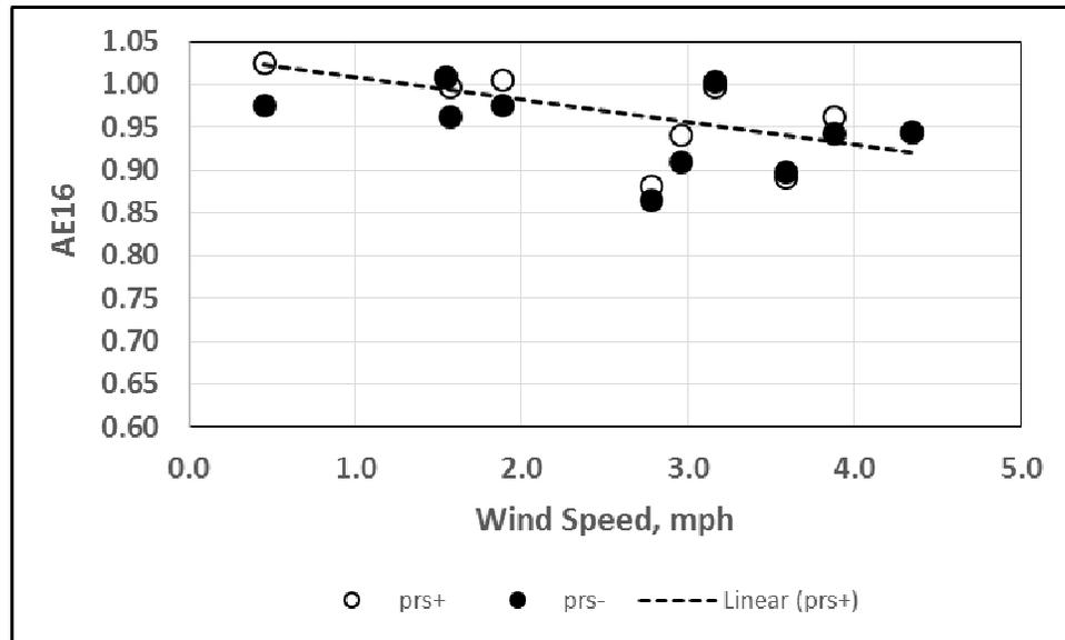
Figure 9. Application efficiency as determined from the 16 internal catch cans (AE16) plotted as a function of wind speed for plots irrigated with prs- and prs+ rotors at system operating pressure of 45psi. Regression lines relating AE16 to wind speed are plotted if the line slopes are significantly different from zero.
