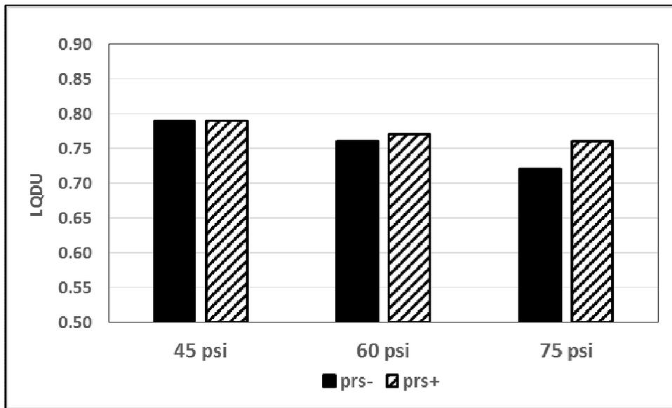
Figure 7. Low quarter mean distribution uniformity (LQDU) for plots irrigated with prs- and prs+ rotors at system operating pressures of 45, 60 and 75 psi.
