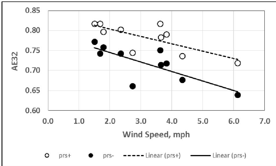
Figure 14. Application efficiency as determined from all 32 catch cans (AE32) plotted as a function of wind speed for plots irrigated with prs- and prs+ rotors at system operating pressure of 75 psi. Regression lines relating AE32 to wind speed are plotted if the line slopes are significantly different from zero.
