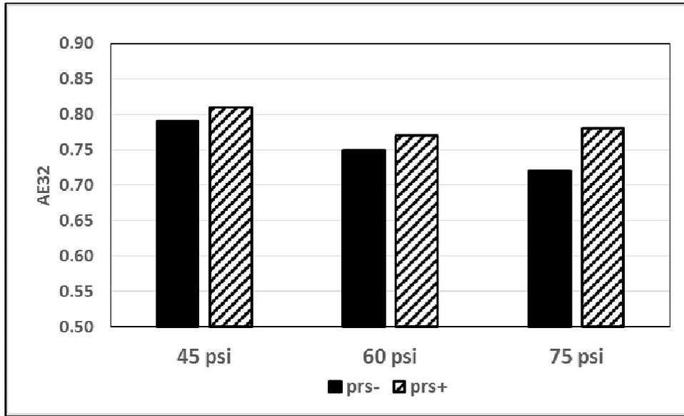
Figure 6. Application efficiency as determined from all 32 catch cans (AE32) for plots irrigated with prs- and prs+ rotors at system operating pressures of 45, 60 and 75 psi.
