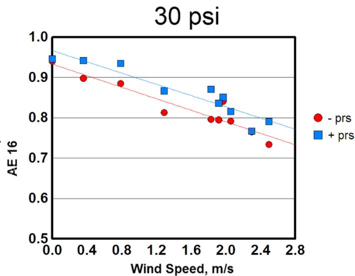
Figure 2. Application efficiency computed using the 16 interior catch cans (AE16) plotted as a function of wind speed during system operation for plots irrigated with (+prs) and without (-prs) pressure regulation when line pressure was set at 30 psi.
