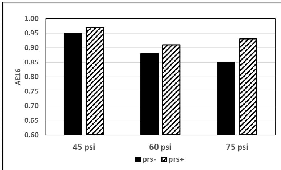
Figure 5. Application efficiency as determined from the 16 internal catch cans (AE16) for plots irrigated with prs- and prs+ rotors at system operating pressures of 45, 60 and 75 psi.
