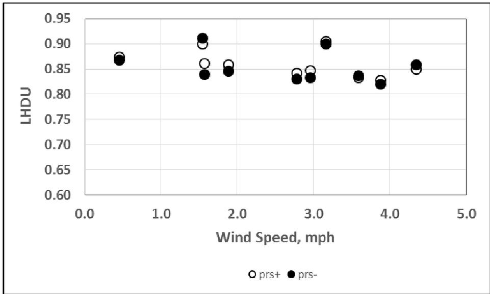
Figure 18. Low half mean distribution uniformity (LHDU) plotted as a function of wind speed for plots irrigated with prs- and prs+ rotors at system operating pressure of 45 psi. Regression lines relating LHDU to wind speed are plotted if the line slopes are significantly different from zero.
