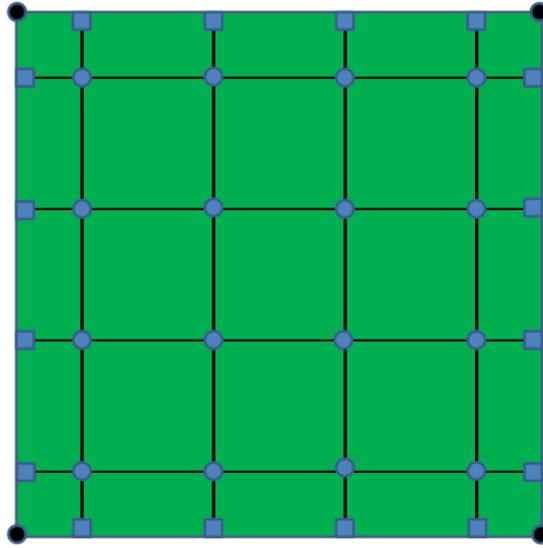
Figure 1. Placement of catch cans on each plot. Blue circles represent interior circular catch cans. Blue squares represent perimeter square catch cans. The separation distance for adjacent circular cans located in the 4x4 matrix was 3.0'.
