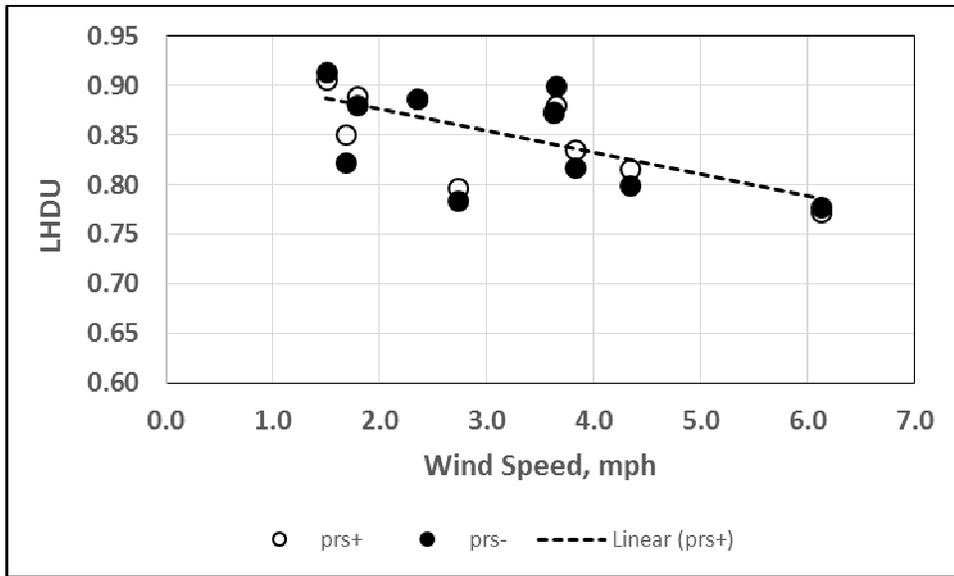
Figure 20. Low half mean distribution uniformity (LHDU) plotted as a function of wind speed for plots irrigated with prs- and prs+ rotors at system operating pressure of 75 psi. Regression lines relating LHDU to wind speed are plotted if the line slopes are significantly different from zero.
