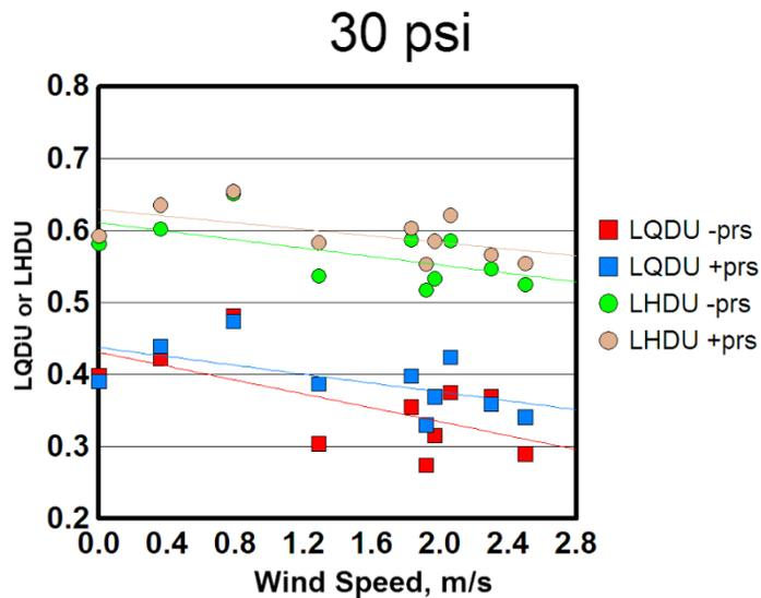
Figure 4. Low quarter distribution uniformity (LQDU) and low half distribution uniformity (LHDU) plotted as a function of wind speed during system operation for plots irrigated with (+prs) and without (-prs) pressure regulation when line pressure was set at 30 psi.
