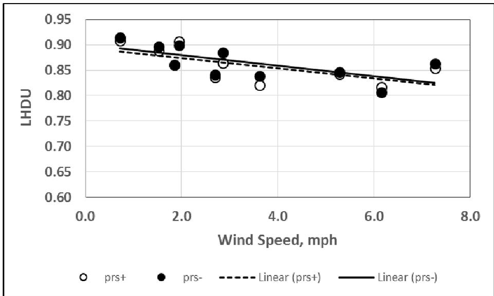
Figure 19. Low half mean distribution uniformity (LHDU) plotted as a function of wind speed for plots irrigated with prs- and prs+ rotors at system operating pressure of 60 psi. Regression lines relating LHDU to wind speed are plotted if the line slopes are significantly different from zero.
