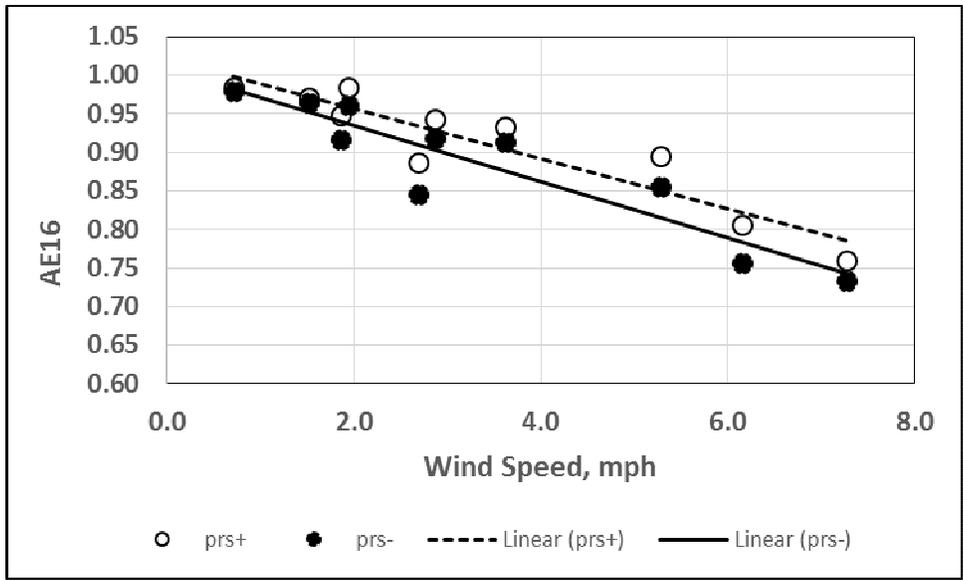
Figure 10. Application efficiency as determined from the 16 internal catch cans (AE16) plotted as a function of wind speed for plots irrigated with prs- and prs+ rotors at system operating pressure of 60 psi. Regression lines relating AE16 to wind speed are plotted if the line slopes are significantly different from zero.
