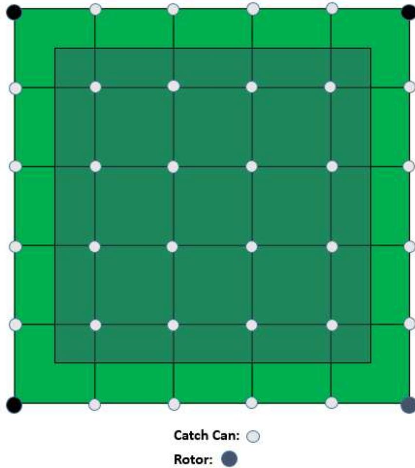
Figure 1. Plot schematic showing the location of the catch cans used to assess irrigation system performance. The 16 internal catch can reside within the darker shaded area.
