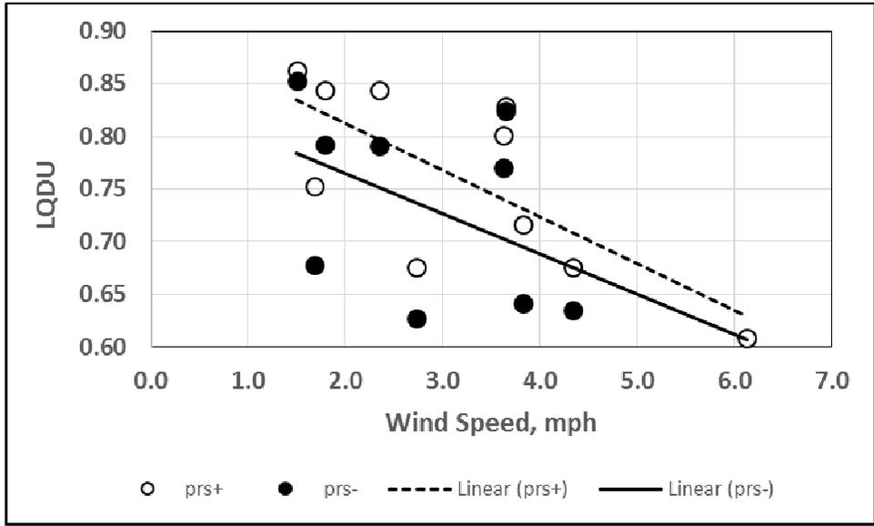
Figure 17. Low quarter mean distribution uniformity (LQDU) plotted as a function of wind speed for plots irrigated with prs- and prs+ rotors at system operating pressure of 75 psi. Regression lines relating LQDU to wind speed are plotted if the line slopes are significantly different from zero.
