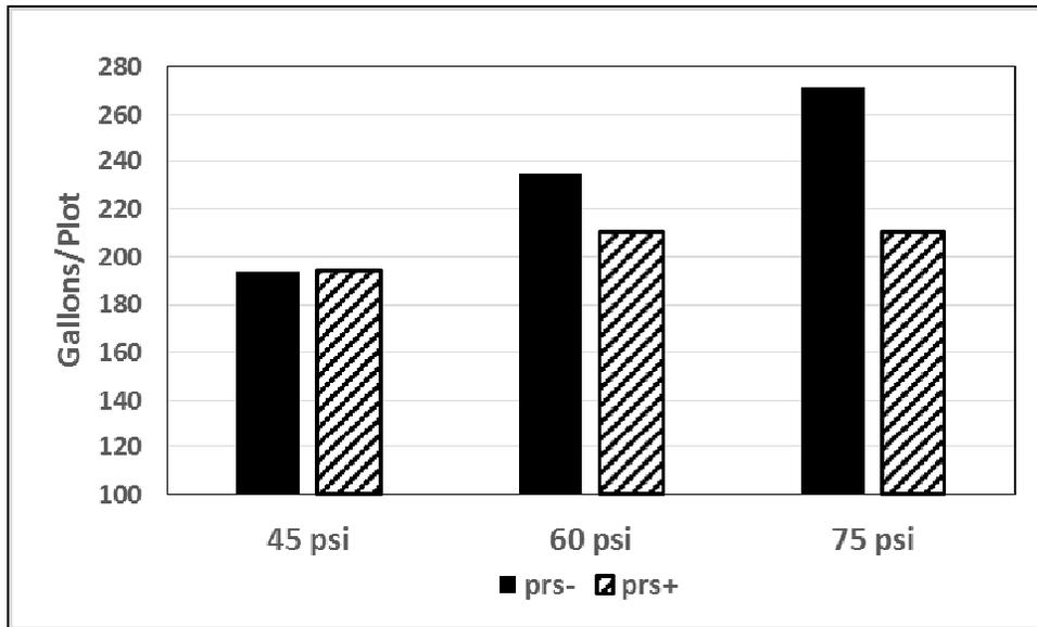
Figure 2. Total volume of water applied to plots irrigated with prs- and prs+ rotors at system operating pressures of 45, 60 and 75 psi.
