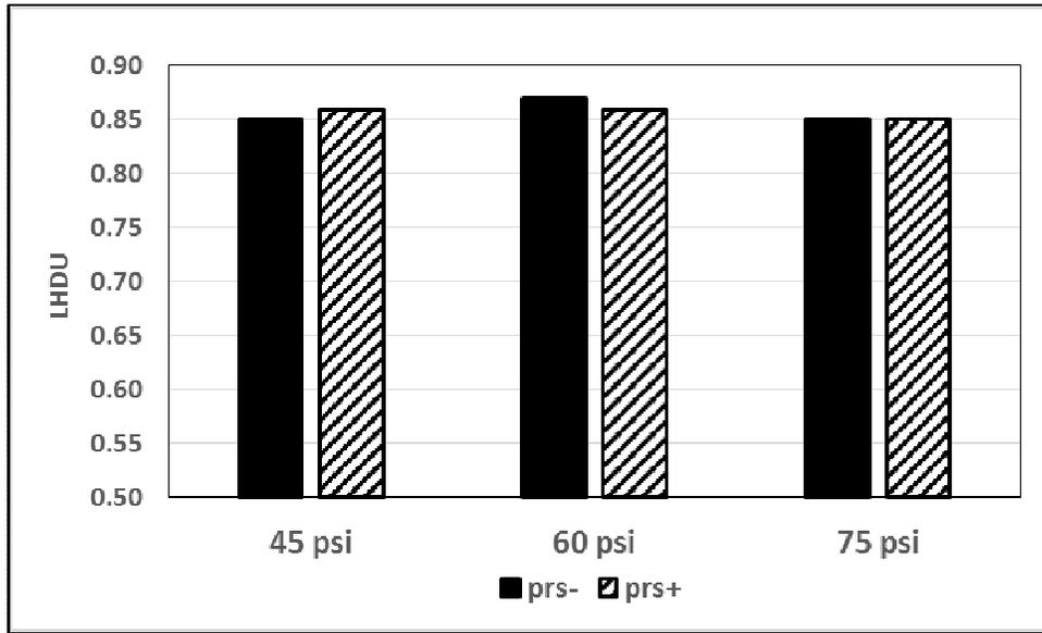
Figure 8. Low half mean distribution uniformity (LHDU) for plots irrigated with prs- and prs+ rotors at system operating pressures of 45, 60 and 75 psi.
