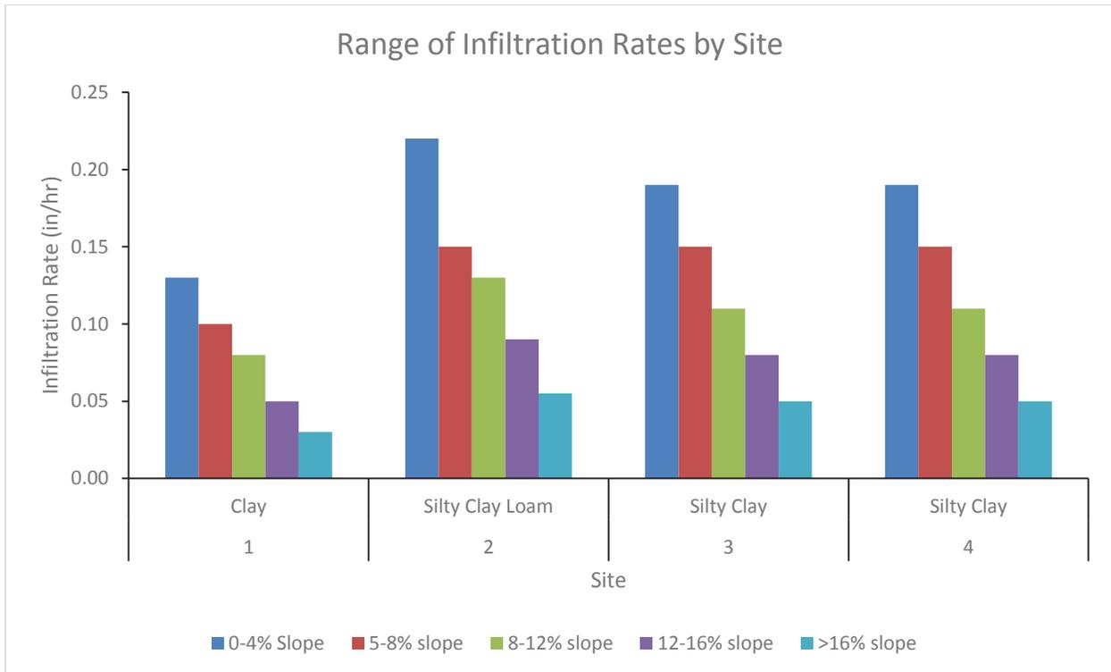
Figure 15. Range of infiltration rates by site (USDA 1990).
