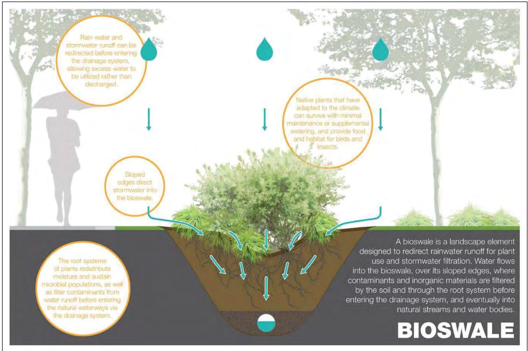
Figure 6. Bioswale graphic replicated from [Upstream Matters](#).
