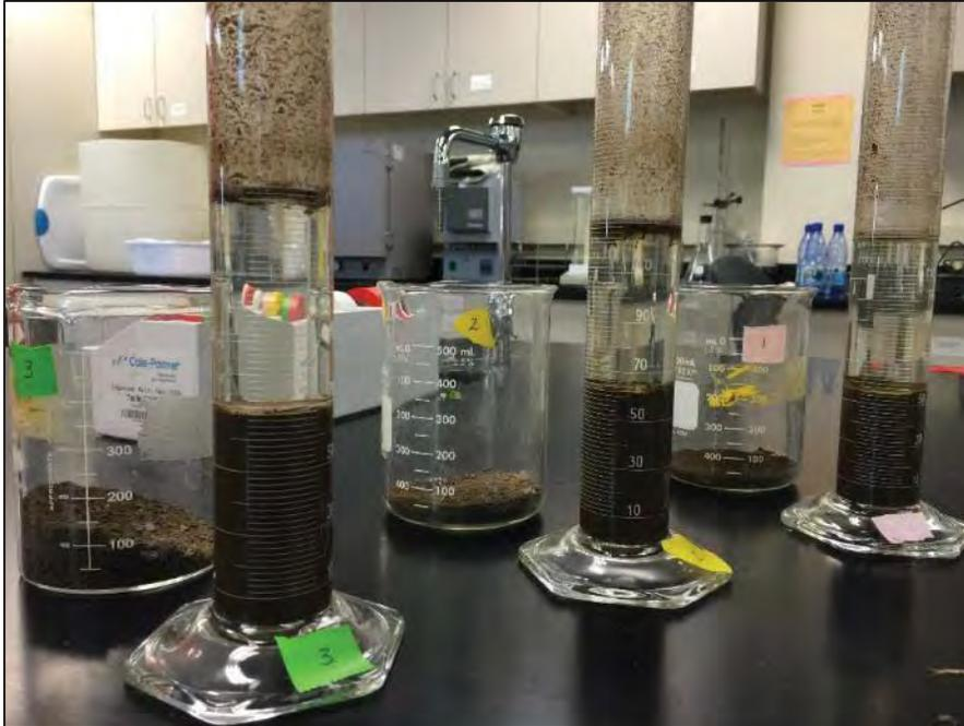
Figure 14. Lab measurement of soil texture from individual rain garden sites.
