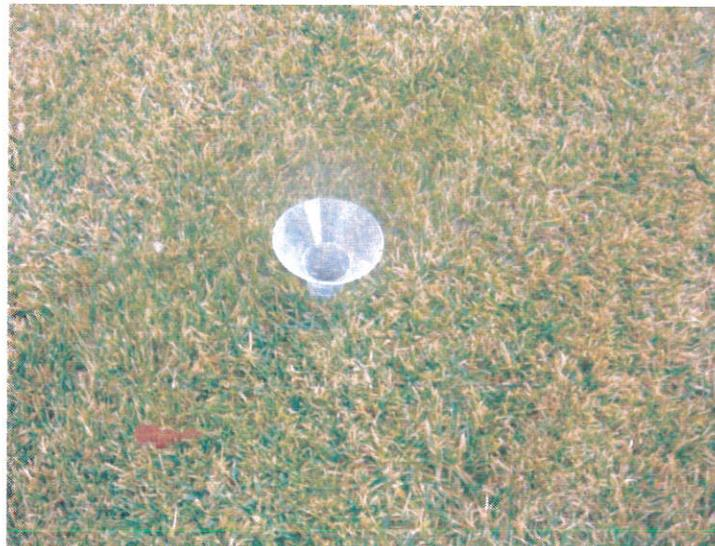
Figure 2. Rain gauge catchment (DWR/Cal Poly)
