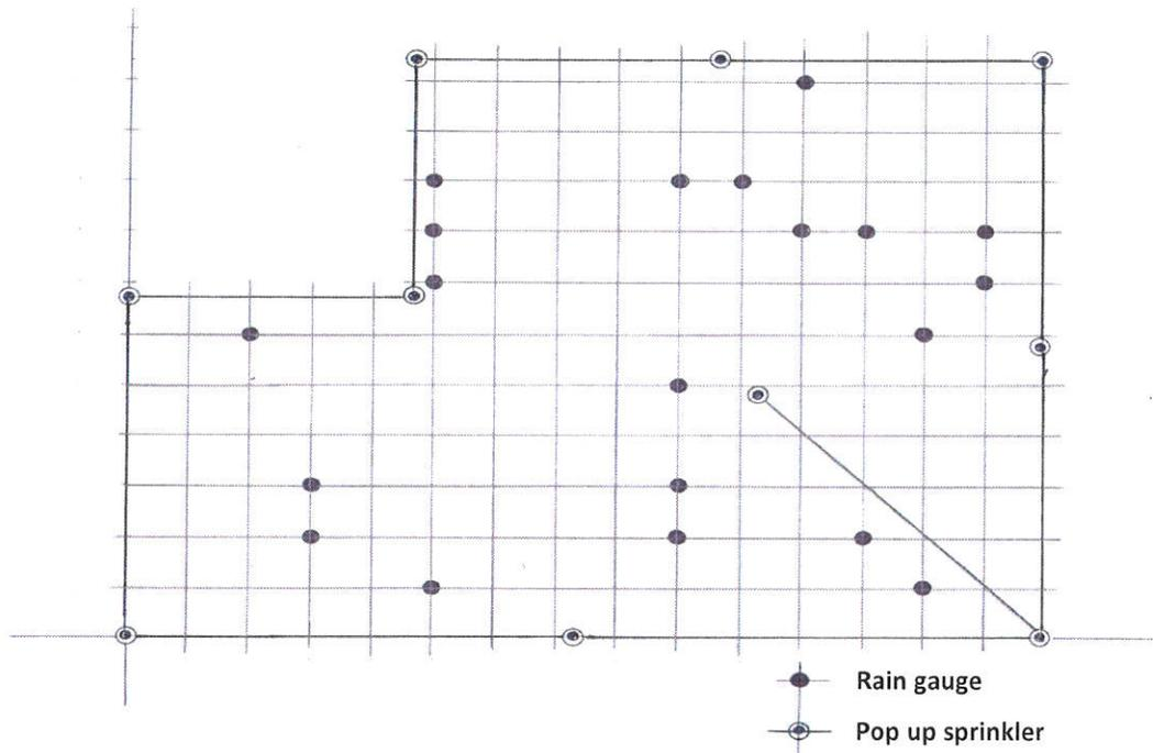
Figure 1. Hydrozone showing randomly located rain gauges and sprinkler locations.
