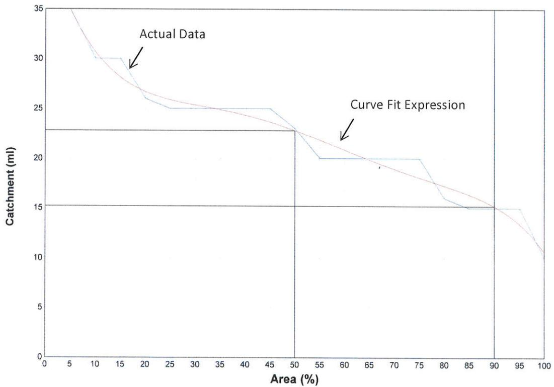
Figure 3. Hydrozone catchment characterization, (ml vs area, %)
