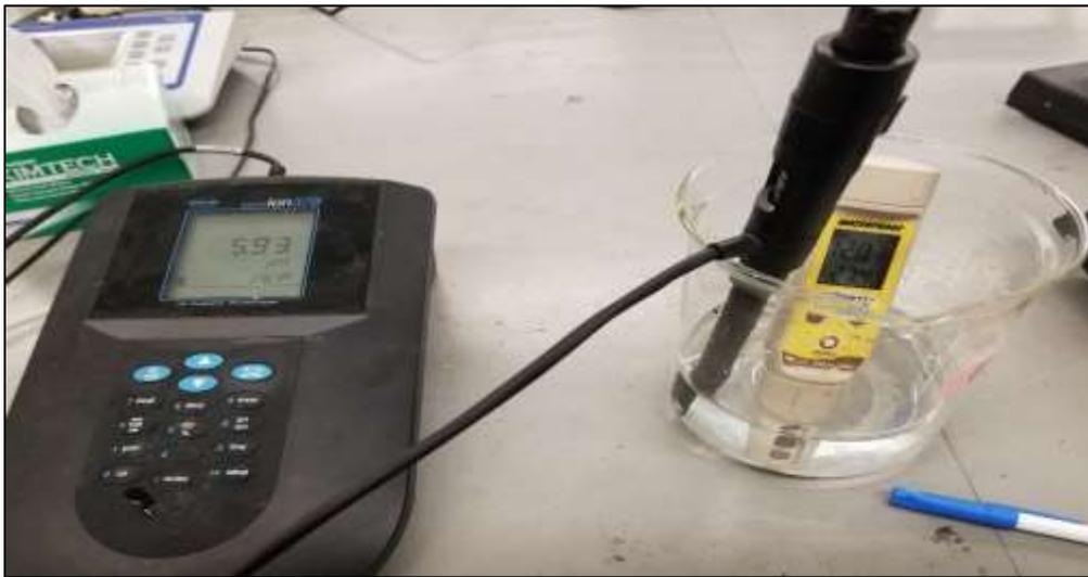
Figure A5. Portable TDS measurement and pH testing
