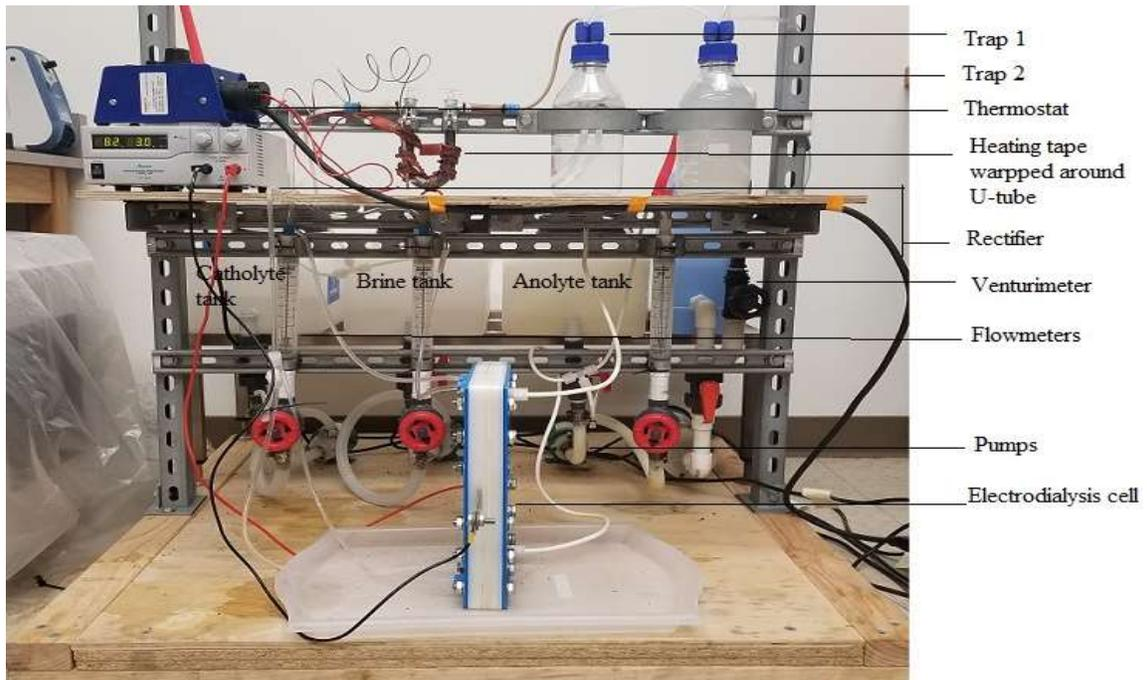
Figure A3. Complete bench-scale setup
