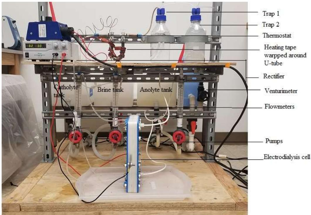
**Figure 2.** Bench scale test kit setup
