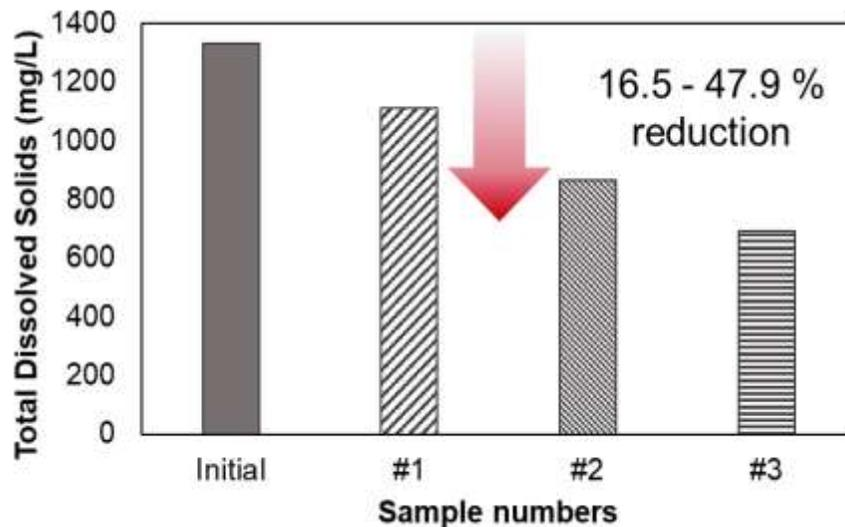
**Figure 3.** The total dissolved solids (TDS) concentrations using 1-chambered cell.
