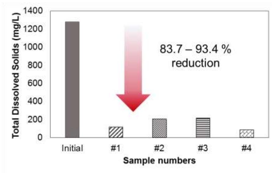
**Figure 4.** The total dissolved solids (TDS) concentrations using 2-chambered cell. Note that sample #4 was treated under a current of 3.5A and other 3 samples (#1-3) under 3.0A with the total operation time of 270 minutes each.
